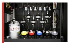
CLEAN AND ERGONOMIC INK SUPPLY SYSTEM 4-liter containers allow for long uninterrupted printing.
