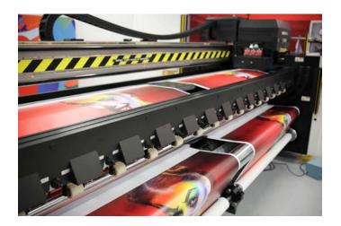
The Oberon RTR3300 comes in a four color plus white and a six color version. The four color plus white version stands out by its ability to print white in different modes. It thus transforms self-adhesive vinyl, static cling or backlit film into vibrant, multi-layered graphics that grab attention.
